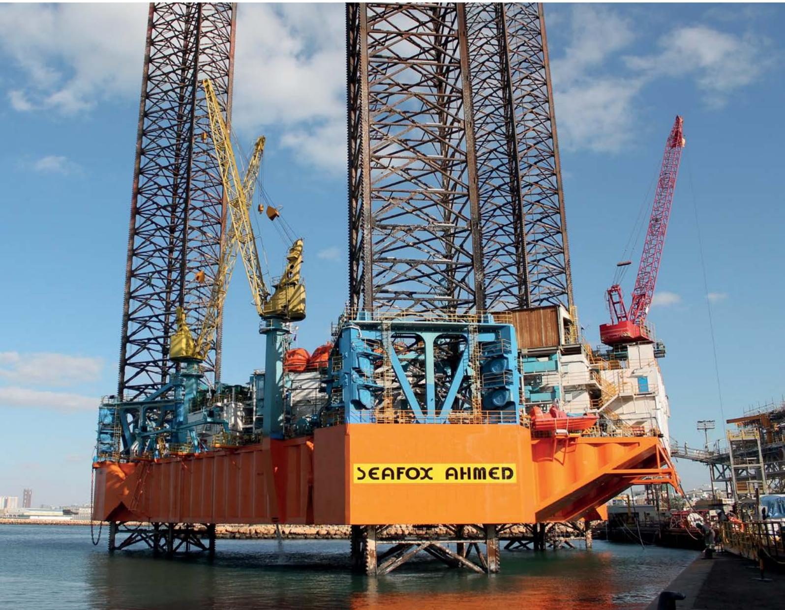
Seafox Ahmed is a three-legged, self-elevating jack-up unit for accommodation and offshore support services built in Vicksburg, Mississippi (USA), by Marathon LeTourneau. She was originally converted to a jack-up ASV in 1993 by Lamprell, in Sharjah, UAE. The last upgrade took place in 2007.
