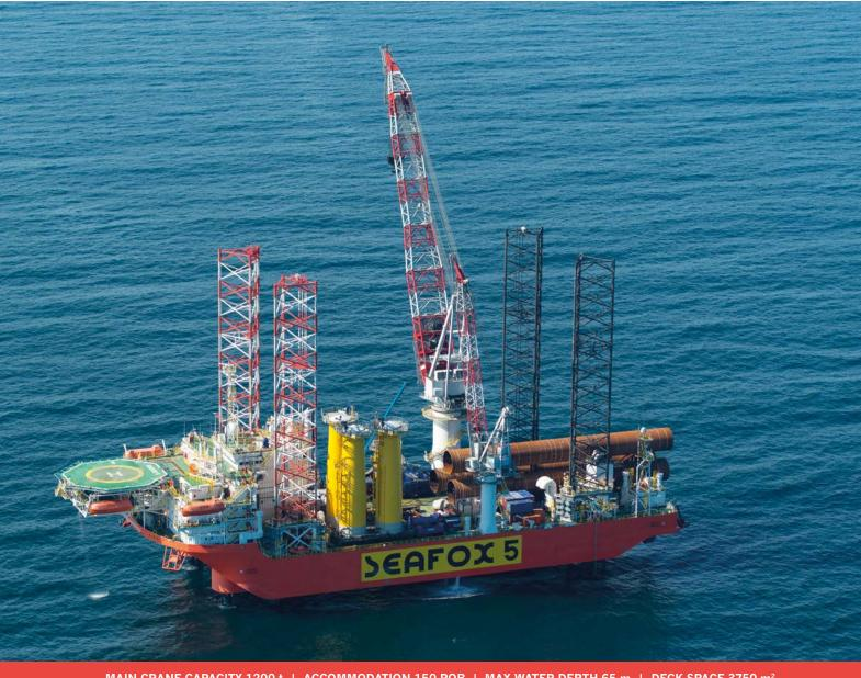
MAIN CRANE CAPACITY 1200 t | ACCOMMODATION 150 POB | MAX WATER DEPTH 65 m | DECK SPACE 3750 m<sup>2</sup>
