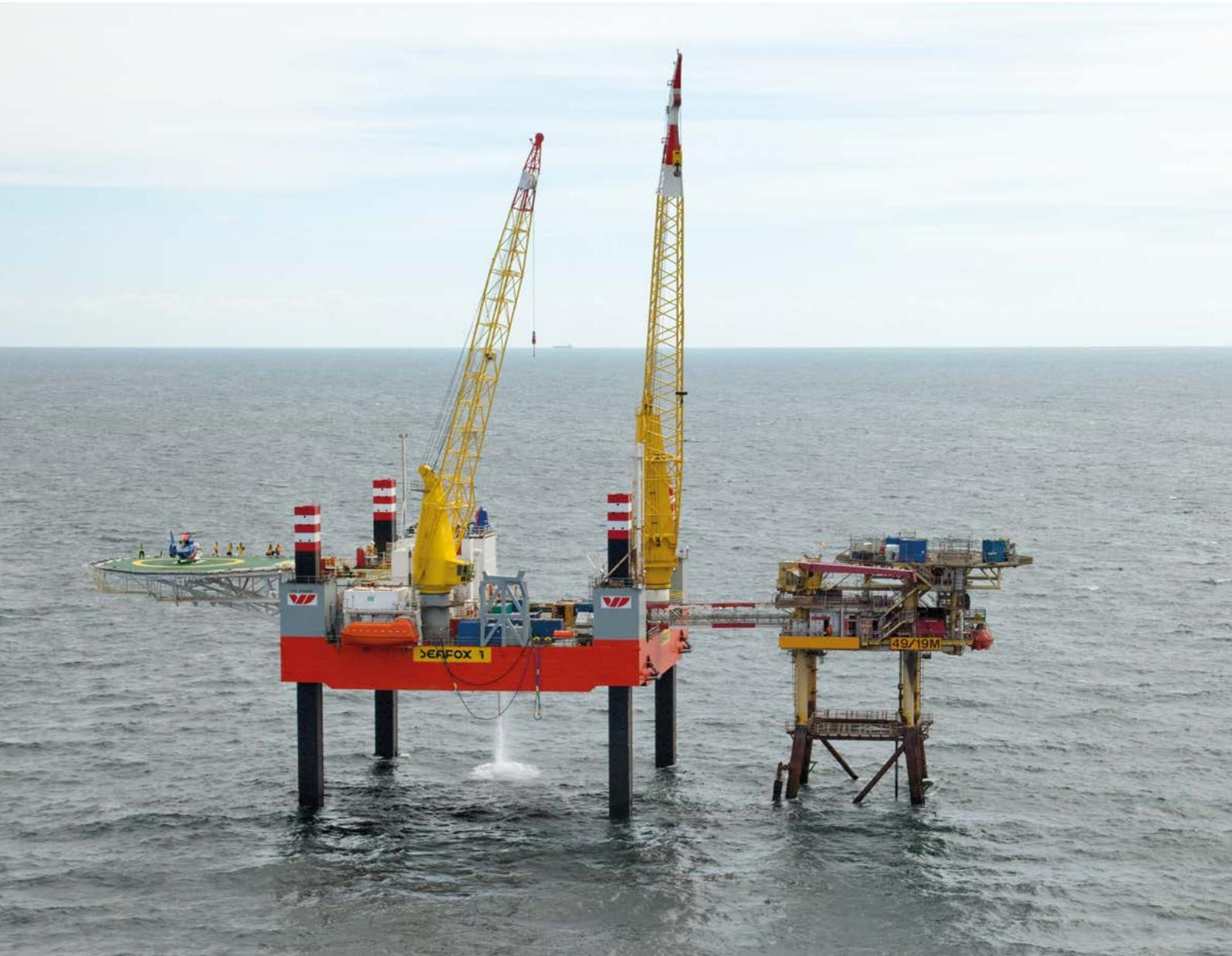
MAIN CRANE CAPACITY 300 t | ACCOMMODATION 75 POB | MAX WATER DEPTH 40 m | DECK SPACE 600 m<sup>2</sup>
